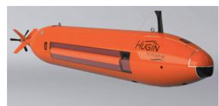
The Norwegian HUGIN large autonomous underwater vehicle - is an autonomous submarine capable of surveillance tasks down to extreme depths (up to 3000m).
